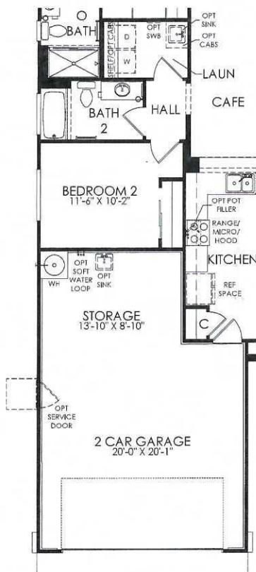
Storage in lieu of Flex This Option Removes Flex and Reduces Livable Square Footage
